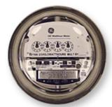
If your meter has 4 or 5 dials as shown here, record the number the dial is pointing towards. When the pointer on a dial is between two numbers, **read the smaller number**. If a dial is too close to tell if it has reached the higher number, *look at the next dial to the right*. If the pointer on that dial has passed zero, then you should record the higher number; otherwise, record the lower number.
