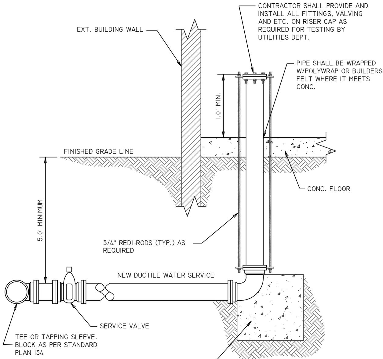
CONTRACTOR SHALL PROVIDE AND INSTALL ALL FITTINGS, VALVING AND ETC. ON RISER CAP AS REQUIRED FOR TESTING BY UTILITIES DEPT.
